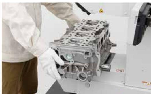
Large workpieces such as cylinder blocks can be mounted on the table as is. Testing of heavy workpieces weighing up to 100 kg is supported.
